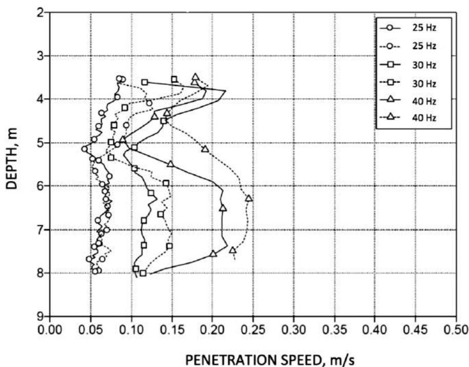
Fig. 16. Sheet pile penetration speed measured at three different vibration frequencies (two tests for each frequency), after [7]
