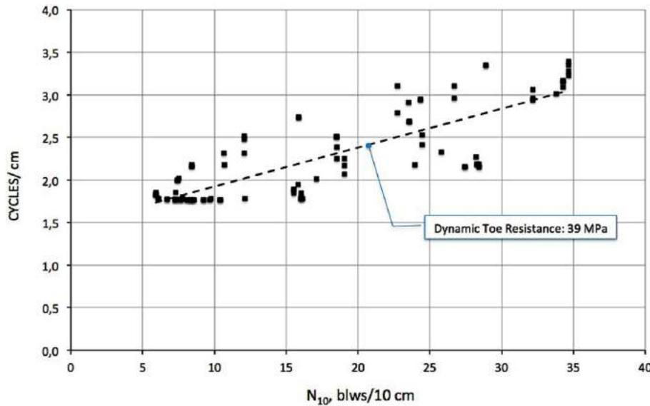
Fig. 17. Relationship between penetration resistance  $N_{10}$  and number of vibration cycles at 40 Hz operating frequency
