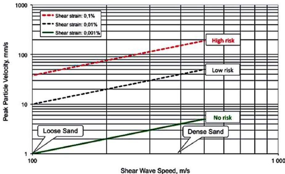
Fig. 18. Assessment of settlement risk in sand as a function of shear wave speed for different shear strain levels [2]
